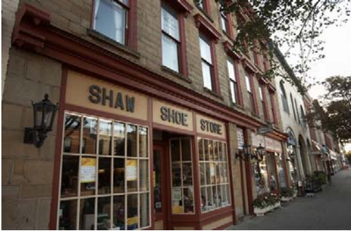
This traditional downtown streetscape exhibits many of the elements that are desirable in downtown Farmingdale. Store facades employ a traditional architectural vocabulary, including inset entrance ways, kick plates below display windows, and the color palette is tastefully composed. Signage is minimally presented and set within a formal sign band above store display windows and hanging signs are appropriately sized so as not to compete with primary signage. The walkway is attractively illuminated with traditional looking wall sconce lighting and other amenities, including planters and outdoor seating areas.
