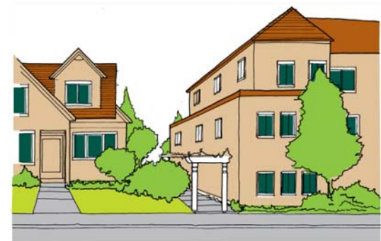
An example of multi-family development that is appropriately scaled to adjacent single-family development. This development also places its parking in the rear, thus preserving the streetscape.
