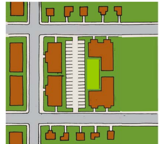
Multi-Family Parking located internally on site between buildings (less desirable).
