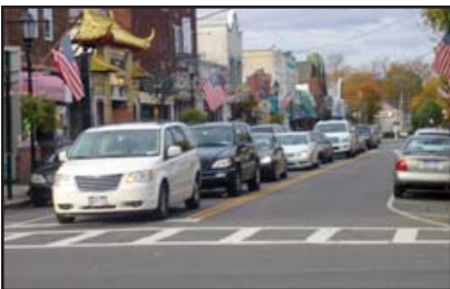
Southbound Main Street traffic is queued behind a vehicle waiting to make a left turn. The single travel lane on Main Street does not permit through traffic to go around a car waiting to complete its left turn. The same condition exists on northbound Main Street.
